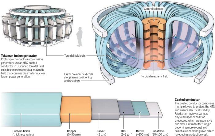
new, largely vapor deposition thin-film production route was needed (*I2*). Notably, Bi-2212 and Bi-2223 can be made by conventional wire fabrication routes but at the price of having poorer texture and consequently lower  $J_c$ . By contrast, industrialization of thin-film CC fabrication processes has resolved both the problem of weak vortex pinning and GB supercurrent obstruction, now enabling mass production of economical HTSs.
